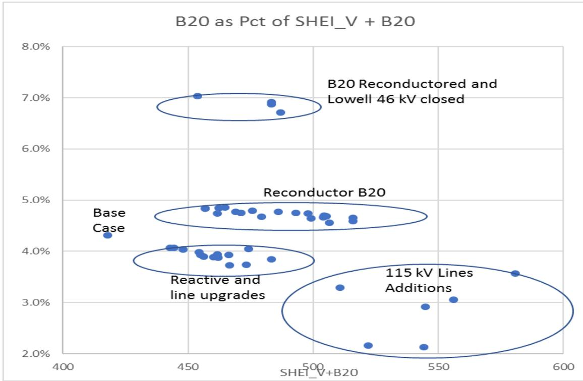
**Figure 16: B20 MW Flow as Percent of SHEI\_V+B20 Flow – All Lines In Cases**
